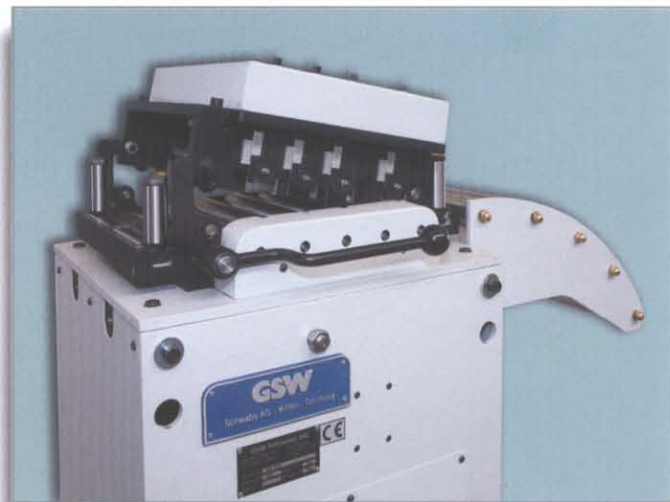
250 mm wide 7-roll Straightener RMA25/74 with manual easy to work head opening.
