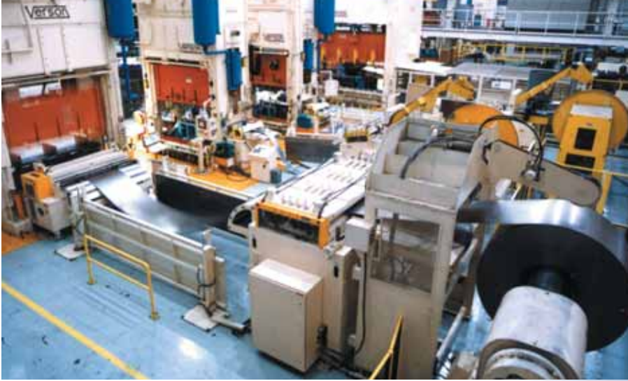
Servo-controlled coil feeding equipment from Coe Press contributes to both quality assurance and production efficiency at Oxford, providing the flexibility to run a variety of parts with fast changeover response to meet Just-In-Time delivery requirements.
