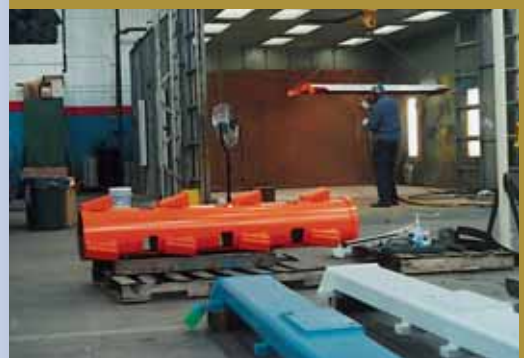
Coe's new 20' x 20' paint booth. The booth was designed to be large enough to handle parts that will be used in Coe and Sesco's large-scale coil feeding systems. Shown in the foreground are finished parts awaiting the next step in the assembly process.
