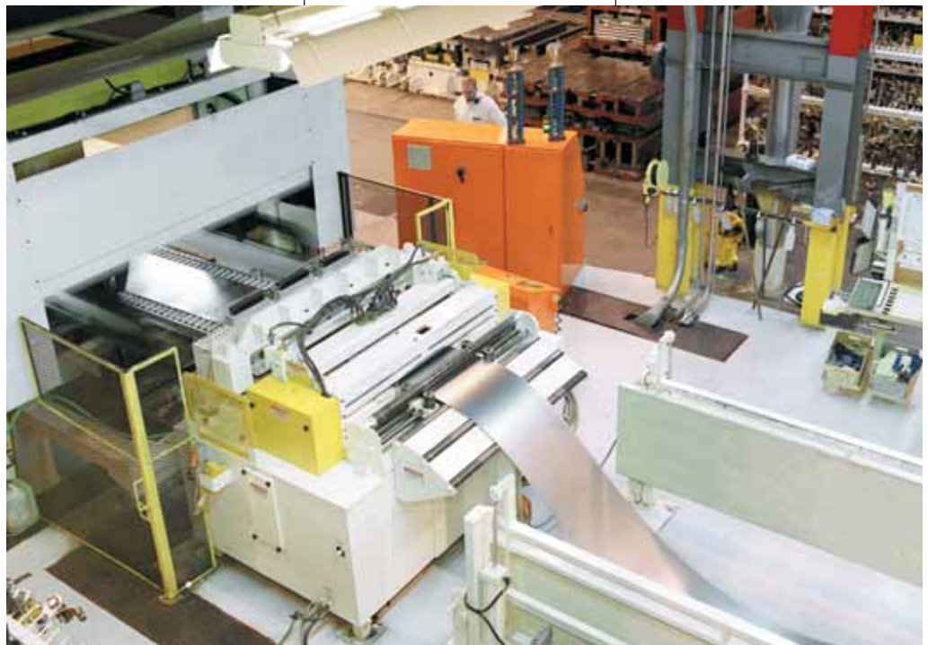
Coe Servo Roll Feed CPRF-560 feeds material into the PTC Combination Link transfer press.
