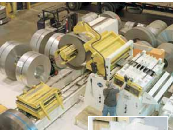
Coe's hydraulic Integral Crop shear used in-line with the coil feeding system allows efficient removal of the "tail hook" when a partially used coil is reversed (backed out) from the press and feeding system and rebanded for future use.
