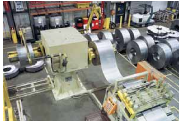
Coe dual mandrel decoiler system helps Shiloh meet the high material demands of high-speed prog die presses, where coil change may occur every 30 minutes.
