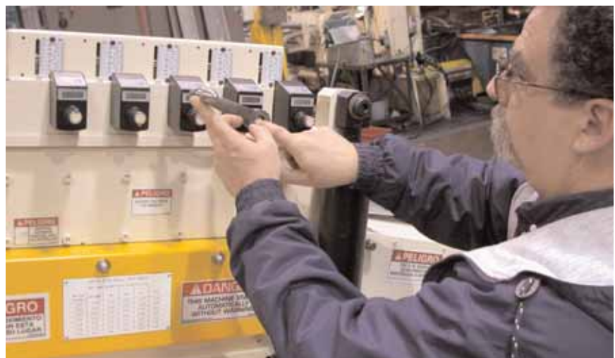
Digital upper straightener roll height indicators help PSS to dial in the exact level settings quickly.
