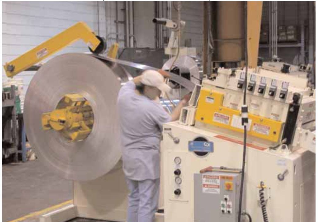
Easy to set up, easy to maintain and clean: Perfection Spring and Stamping operates this precision 11 roll power straightener and pulloff reel combination.
