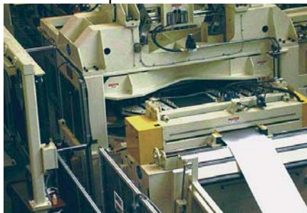
"Square cut or trapezoidal shaped blanks are produced at a rate of 30/minute via this oscillating shear die, feeding downstream progressive die operations"
