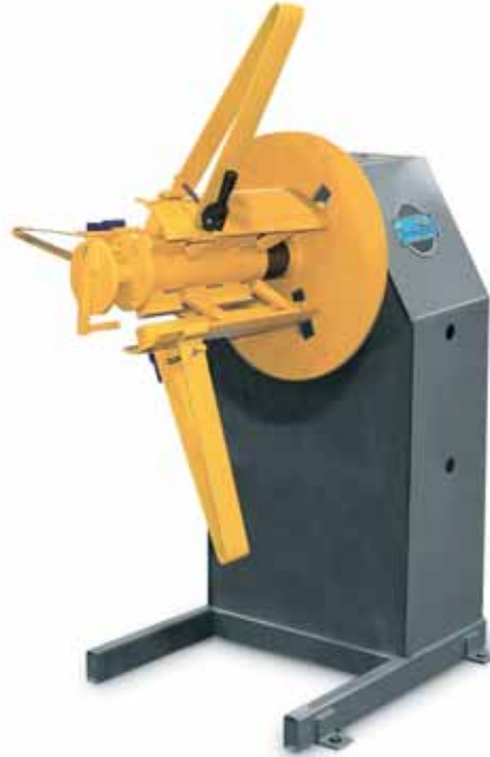
■ Standard 2,500# Series reel configured for "pull-off" application with manual hand crank expansion with a snapout handle, and a 30" diameter heavy duty backplate.
